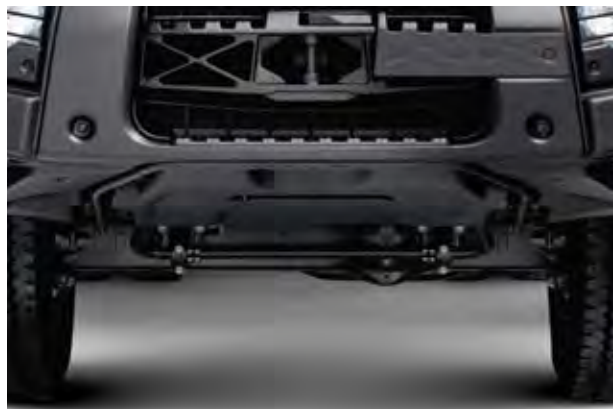
GUARD PLATE underneath the radiator and oil sump.
